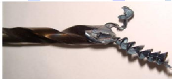
Fig.2. chips welded on cutting edges.
