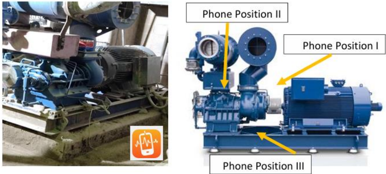
Figure 7: Vibration measurements with a Phyphox App Vibration analyzer.
