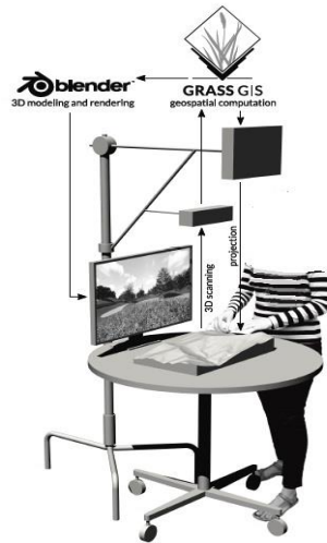
Figure 4. Tangible Landscape: a real-time cycle of 3D scanning, geospatial computation and 3D modeling, and projection and 3D rendering [9]
