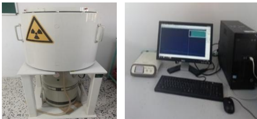
Figure 3. High purity Germanium detector (HPGe) P-Type (Centre of Radiation Measurements and Training).
