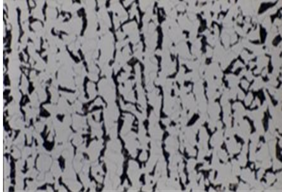
Figure1. Optical micrograph of microstructure of the carbon steel original starting material, 200X.
