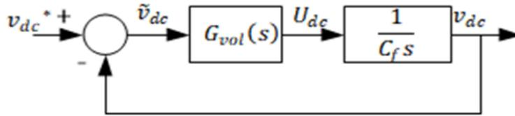
Figure 4: DC voltage Control Loop
