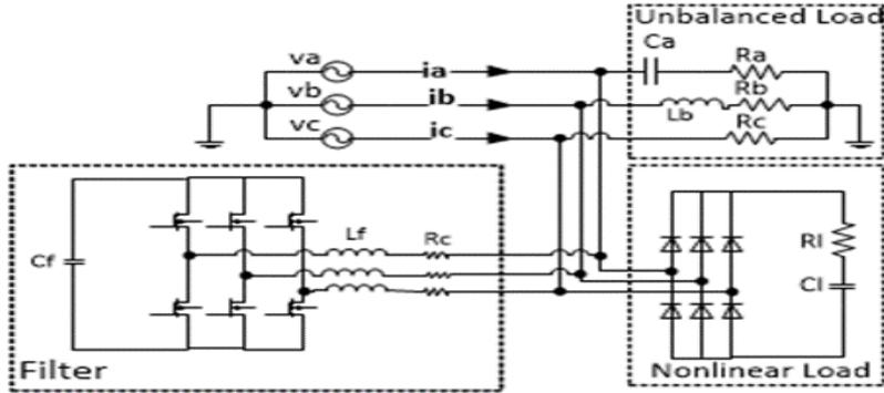
Figure 1: System Configuration
