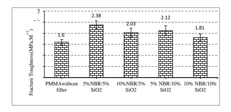
Figure 4. Fracture toughness of PMMA denture base reinforced with NBR/SiO<sub>2</sub> particles compared to unreinforced PMMA material.
