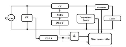
Figure 3: Schematic diagram of the APFC system
