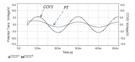
Figure 8: Voltage and current waves of the supply after correction for  $6{+}j8\Omega \;load$
