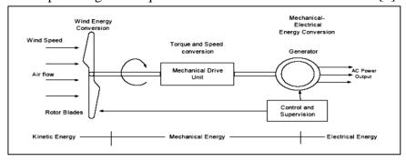
Figure 2. Power transfer in a wind energy converter
