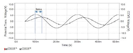
Figure 6: Voltage and current waves of the supply before correction for 6+j8 load
