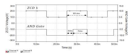
Figure 5: ZCD-1 & AND Gate outputs before correction for  $6+j8\Omega$  load
