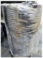
Figure 9. GFRP rupture
