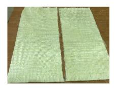
Figure 2. Tyfo SEH-51A Composite Uni-directional Glass Fiber
