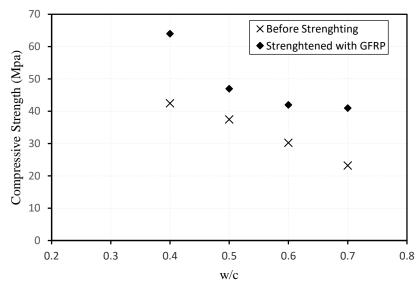
Figure 12. Compressive strength- water cement ratio curve results – "GFRP Specimens"
