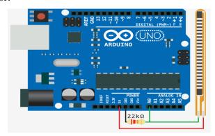
Figure 10 Arduino Uno with the flex sensor
