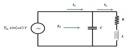
Figure 1: Load and capacitor connected in parallel
