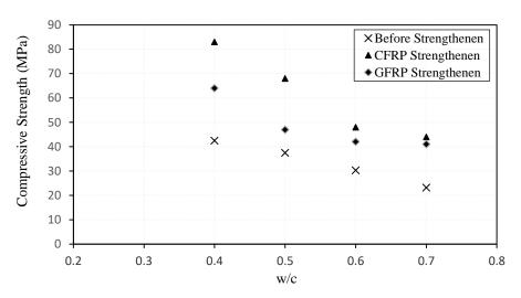
Figure 13. Compressive strength- water cement ratio curve results "CFRP and GFRP specimens"
