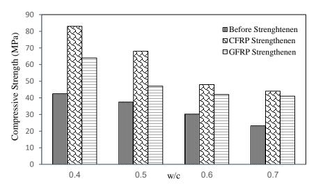
Figure 14. Compressive strength- water cement ratio results – "CFRP and GFRP Specimens"
