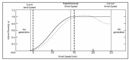
Figure 3. Typical curves for a constant speed, stall-controlled (dotted) and variable speed pitch controlled (solid) wind turbine
