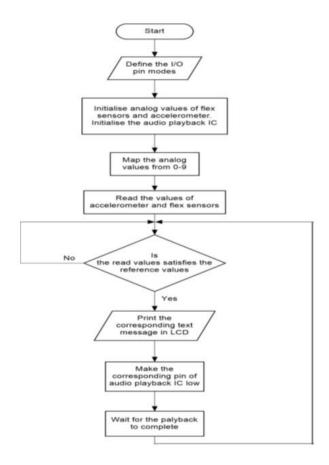
Figure 9 Flowchart of the software implementation
