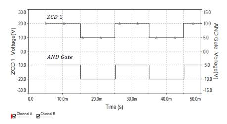
Figure 7: ZCD-1 & AND Gate outputs after correction for  $6+j8\Omega$  load
