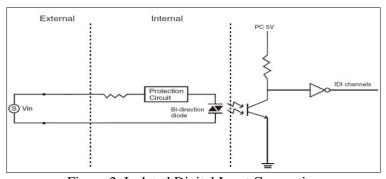
Figure 2. Isolated Digital Input Connection
