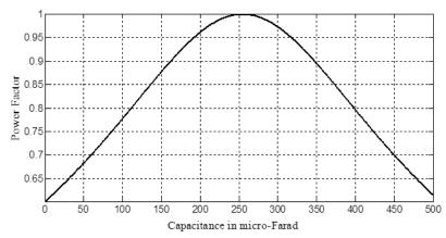
Figure 2: Power factor versus capacitance
