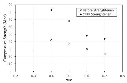
Figure. 11. Compressive strength- water cement ratio curve results – "CFRP Specimens"
