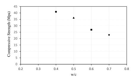
Figure. 8. Compressive strength- water cement ratio Curve Results – "original Specimens"
