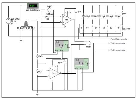
Figure 4: Simulation of the APFC system
