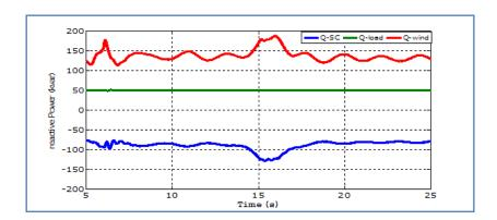
Figure 11. The diesel system's and wind energy system's reactive power variations
