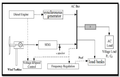
Figure 8. Block diagram of the hybrid generation system
