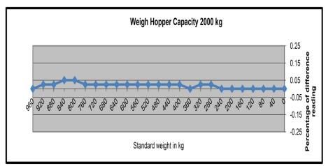
Figure 6. Percentage of scale error reading differences (calibration certificate -2019).
