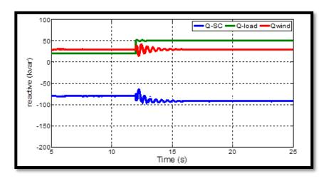
Figure 16. The hybrid system's reactive power with load variations
