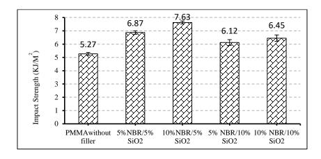
Figure 3. Impact strength of PMMA denture base reinforced with NBR/SiO<sub>2</sub> particles compared to unreinforced PMMA material.
