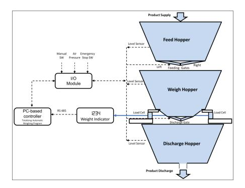
Figure 1. The components of the proposed bulk weighing system
