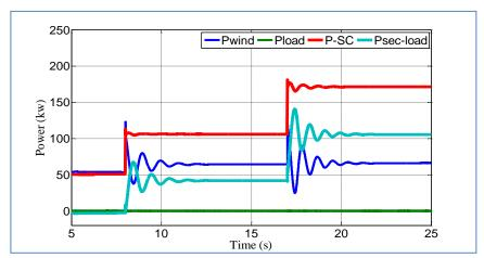
Figure 15. The diesel and wind energy system's real power output with load variations
