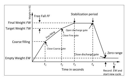
Figure 5. Sequential Operation for one cycle
