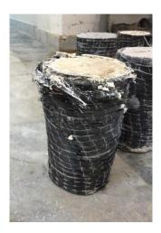
Figure 10. CFRP delamination failure
