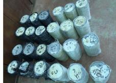
Figure 5. Glass Fiber wrapping for Cylindrical Column
