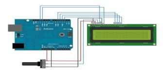
Figure 12 Arduino Uno with LCD
