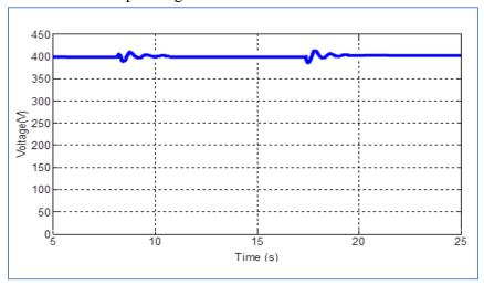
Figure 17. The hybrid system's voltage at load terminals
