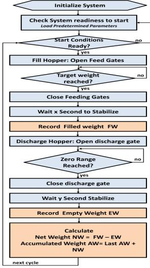
Figure 4. Weighing operation sequence
